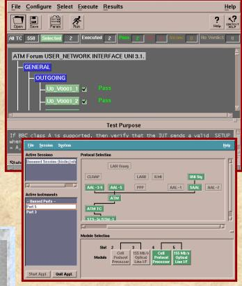
The project involves the development of a flexible, efficient and inexpensive analyser card and related test software. The analyser card provides an OC-3C interface to connect to an ATM network. The software provides flexible ways to operate the analyser card, analyse the raw captured data and calculate the QoS parameters.
