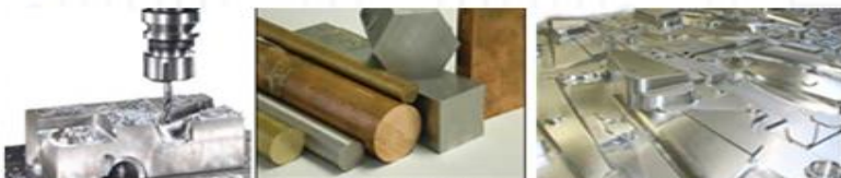
Fig 2.5: Removing unwanted materials from the original blocks to form the desired shapes with specific functions.
