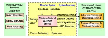
Figure 4. Boundary setting for metrics modeling of waste-to-material recovery processes.
