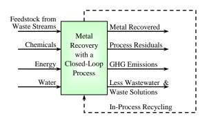
Figure 12. A closed-loop metal recovery process with in-process recycling.
