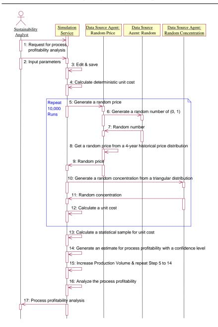
Figure 8. Sequence diagram for probabilistic analysis of process profitability.
