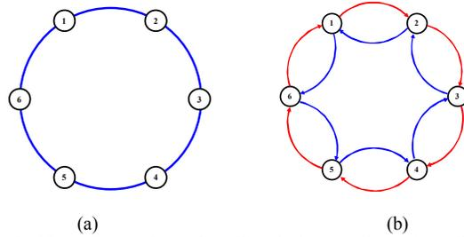
Fig. 2: Network topology for all-optical networks: (a) undirected graph, and (b) directed graph. Each undirected link in the undirected graph is replaced by two directed arcs in opposite directions, to illustrate bidirectional connections between adjacent nodes.
