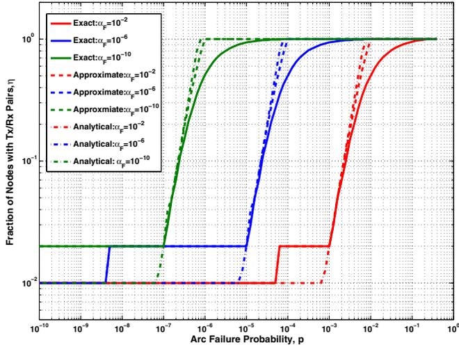
Fig. 5. The required fraction of nodes with Tx/Rx pairs for different target cumulative diagnosability probabilities is plot against the arc failure probability. They share similar “S” shapes.
