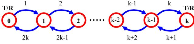
Fig. 3. The canonical linear network with  $k+1$  nodes and  $2k$  arcs: nodes at both ends are equipped with diagnostic Tx/Rx pairs.
