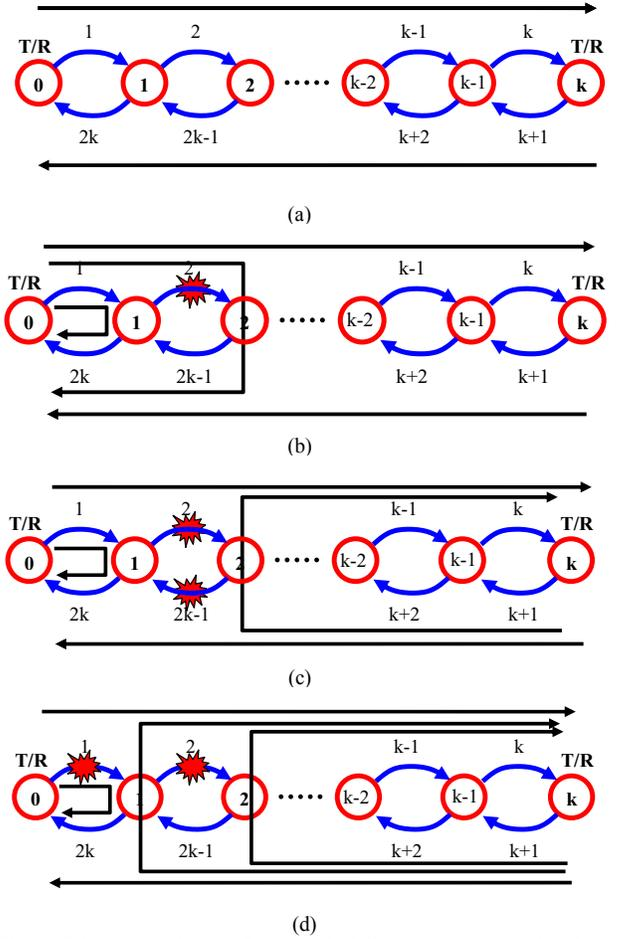
Fig. 4. Diagnosis schemes for canonical linear networks under three types of diagnosable failure patterns: (a) failure pattern with zero arc failure, (b) failure patterns with single arc failure, (c) failure patterns with two arc failures in both directions of one bidirectional link and (d) failure patterns with two arc failures in two consecutive arcs in the same direction.
