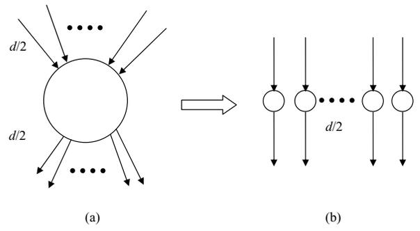
Fig. 7. Node replication approach: (a) a node of degree  $d$  has  $d/2$  in degree and  $d/2$  out degree, (b) the node is replicated with  $d/2$  virtual nodes, each of which has 1 in degree and 1 out degree.
