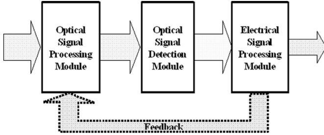
Fig. 3. Structured receiver architecture. It is divided into three cascaded modules: an optical signal processing module, an optical detection module, and an electrical signal processing module.
