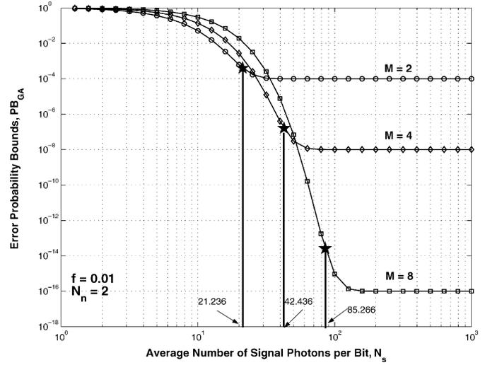
Fig. 5. Error probability bounds for the idealized receiver with different number of lightpaths.  $f = 0.01$  and  $N_n = 2$ .
