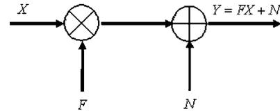
Fig. 2. Discrete channel model of an individual lightpath.  $X$  is the input,  $Y$  is the output,  $F$  is a Bernoulli random variable indicating the lightpath state, and  $N$  is the noise.
