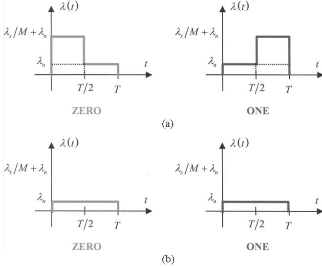
Fig. 4. Detected photo-event rates for two hypotheses with BPPM signaling. (a) When the lightpath is UP, the detected rate is the sum of the signal rate and the noise rate. (b) When the lightpath is DOWN, the detected rate is only the noise rate.
