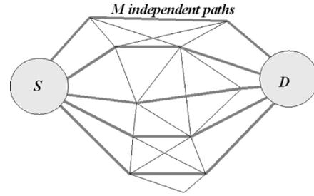
Fig. 1. Network model for an  $M$ -connected source-destination pair in a densely connected all-optical network.
