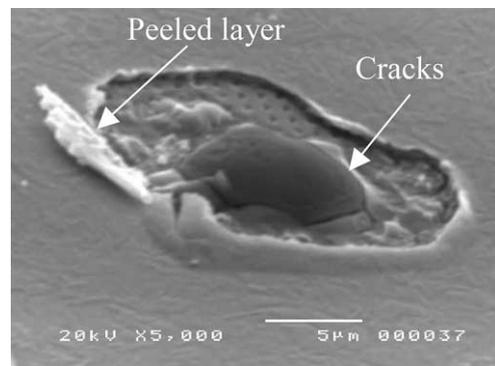
Fig. 6. Etched bond pads on the low- $k$  device bonded with type-3 wire.
