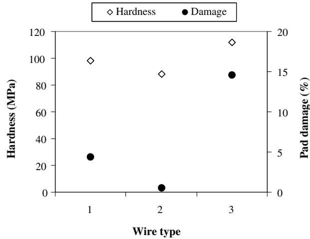
Fig. 3. Bulk hardness and pad damage in percentage.
