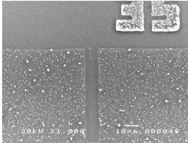
Fig. 7. Etched bond pads on the base-lined SiO<sub>2</sub> device bonded with type-3 wire.
