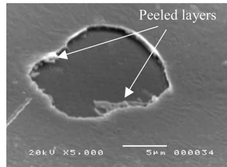
Fig. 5. Etched bond pads on the low- $k$  device bonded with type-1 wire.
