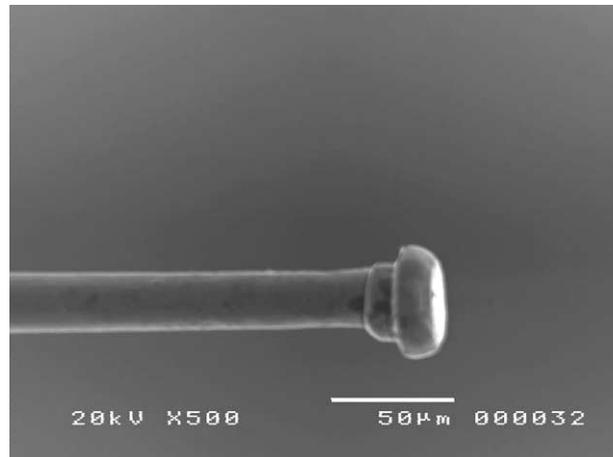
Fig. 2. SEM picture of a squashed FAB.
