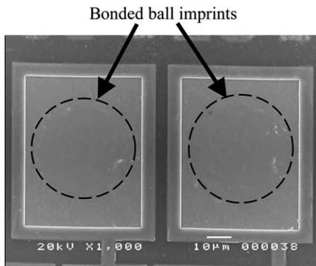
Fig. 4. Etched bond pads on the low- $k$  device bonded with type-2 wire.
