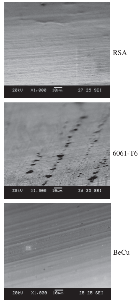
Fig. 3. SEM micrographs of the spherical concave surfaces of the three mold inserts machined using the ultra-precision turning machine.
