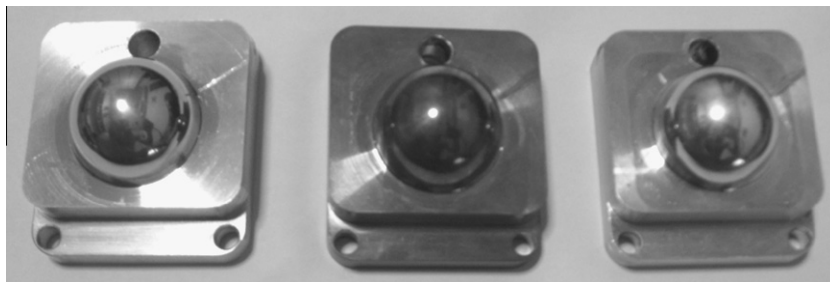
Fig. 1. Core inserts with spherical convex surfaces machined using a CNC turning machine.
