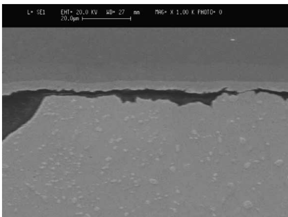
Fig. 5. SEM picture with a high magnification showing a crack after 3000 thermal cycles (0.2-mm stencil thickness, 250 °C reflow, 0.56-mm pad size).
