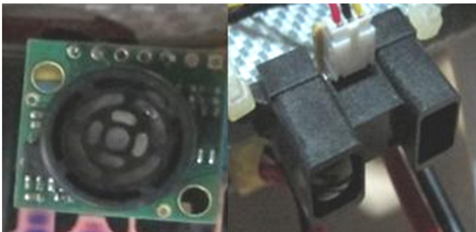
Fig. 4. Ultrasonic and infra-red range finders used.
