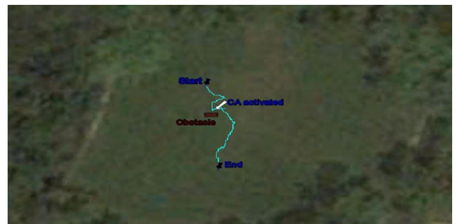
Fig. 23. Trajectory of the UAV during navigation and collision avoidance.
