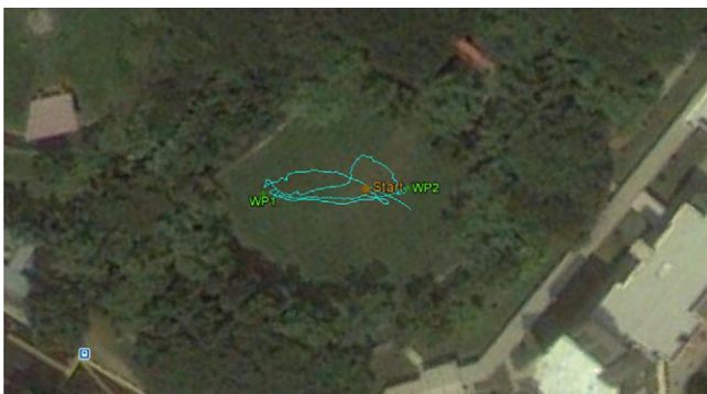
Fig. 18. Autonomous waypoint navigation with two waypoints.
