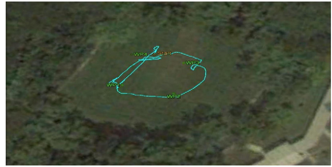
Fig. 19. Autonomous waypoint navigation with four waypoints.
