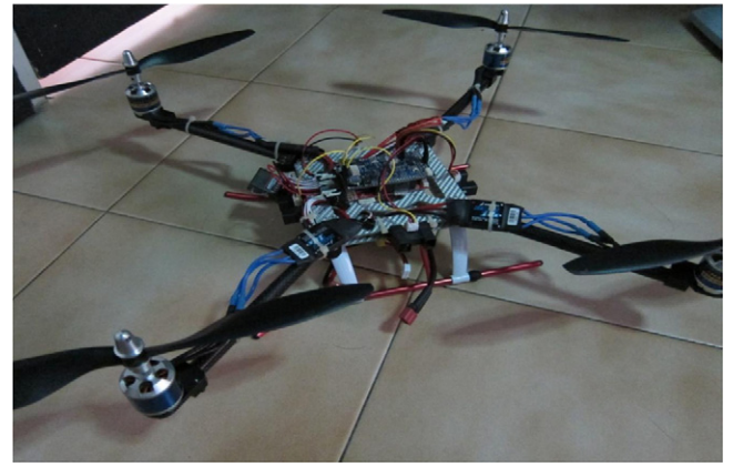
Fig. 1. Integrated quadrotor platform with flight controller, sensors and propulsion.
