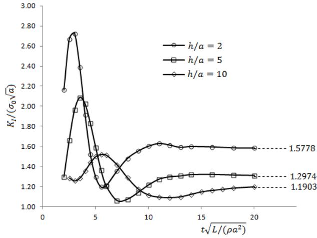
Figure 5. Plots of  $K_I/(\sigma_0\sqrt{a})$  at an inner crack tip against  $t\sqrt{L/(\rho a^2)}$  for  $d/a = 0.50$  and selected values of  $h/a$ .
