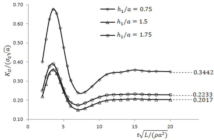
Figure 11. Plots of  $K_{II}/(\sigma_0\sqrt{a})$  against  $t\sqrt{L/(\rho a^2)}$  for  $h/a = 4.0$  and selected values of  $h_1/a$ .
