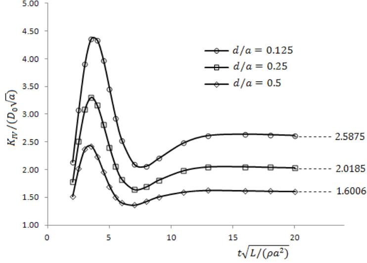
Figure 8. Plots of  $K_{IV}/(D_0\sqrt{a})$  at an inner crack tip against  $\sqrt{L}/(\rho a^2)$  for  $h/a = 4.0$  and selected values of  $d/a$ .
