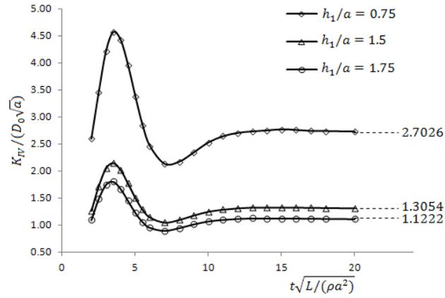
Figure 12. Plots of  $K_{IV}/(D_0\sqrt{a})$  against  $t\sqrt{L}/(\rho a^2)$  for  $h/a = 4.0$  and selected values of  $h_1/a$ .
