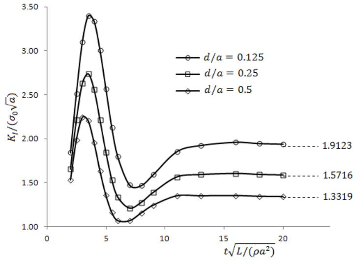
Figure 7. Plots of  $K_I/(\sigma_0\sqrt{a})$  at an inner crack tip against  $\sqrt{L/(\rho a^2)}$  for  $h/a = 4.0$  and selected values of  $d/a$ .
