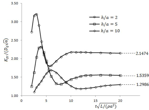
Figure 6. Plots of  $K_{IV}/(D_0\sqrt{a})$  at an inner crack tip against  $t\sqrt{L/(\rho a^2)}$  for  $d/a = 0.50$  and selected values of  $h/a$ .
