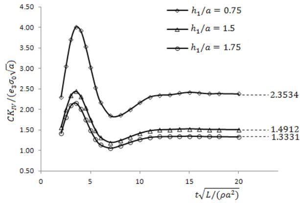
Figure 13. Plots of  $CK_{IV}/(e_3\sigma_0\sqrt{a})$  against  $t\sqrt{L}/(\rho a^2)$  for  $h/a = 4.0$  and selected values of  $h_1/a$ .
