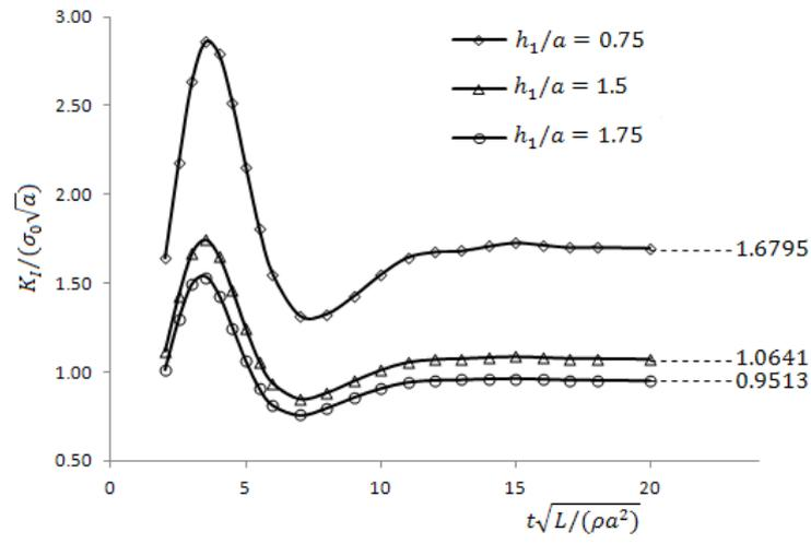
Figure 10. Plots of  $K_I/(\sigma_0\sqrt{a})$  against  $t\sqrt{L/(\rho a^2)}$  for  $h/a = 4.0$  and selected values of  $h_1/a$ .
