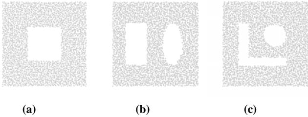
**Figure 16: Network settings.** (a) Basic setting, 5376 nodes (average degree = 12.9); (b) Two holes, 4697 nodes (average degree = 12.9); (c) Two holes (one concave), 5142 nodes (average degree = 12.8).
