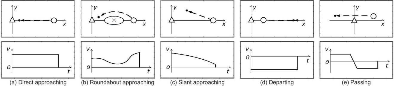
**Figure 3: Five categories of relative trajectories (the upper row) and their corresponding Doppler profiles (the bottom row). One person (in triangle) is fixed in the axis origin. The relative movement of the other person (in circle) is depicted in a dashed line.**
