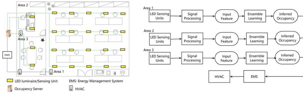
**FIGURE 2.** System architecture of VLS based occupancy inference.
