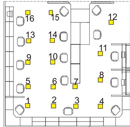
FIGURE 4. Sensing units layout in CeilingSee testbed [13].
