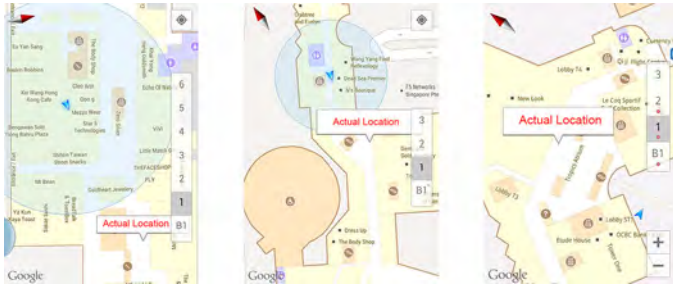
(a) Screenshots for GMI. The blue arrows indicate locations estimated by GMI and the labels show the actual location. Though without actual measurements, the differences between the estimated and actual locations are clearly very significant.
