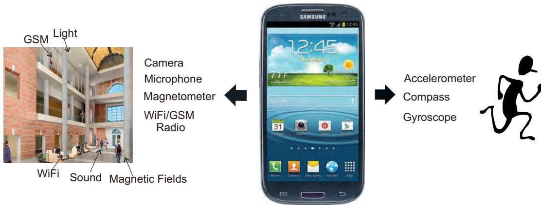
Fig. 1. Location inference using smartphone sensors: fingerprinting (FP) is performed through built-in sensors indicated on the left side, whereas dead reckoning (DR) is performed through sensors on the right.
