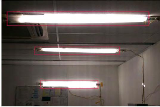
Fig. 8. CeilingCast testbed: three LED luminaires are mounted on wall and ceiling with an interval of 1.5m, and the ceiling is 2.5m above the floor.
