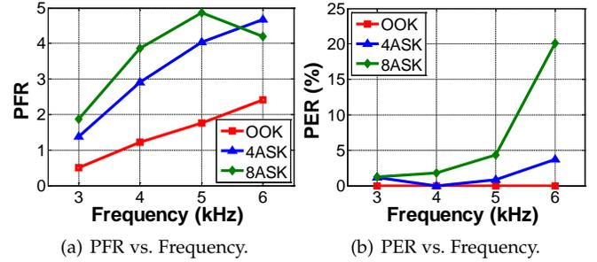
Fig. 9. PFR and PER with a varying transmission frequency.
