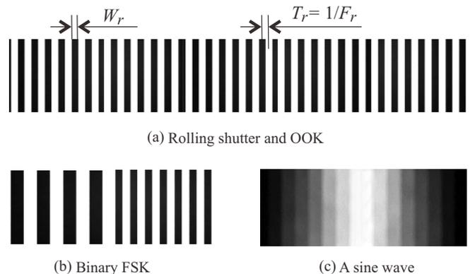
Fig. 1. Illustrating rolling shutter and modulations. (a) When setting  $F_m = F_r$ , the time lapse between sampling two brands is exactly  $1/F_r$ , and the width of each band is  $W_r$ . (b) BFSK constructed by two OOKs with different frequencies. (c) A sine wave sampled by rolling shutter.
