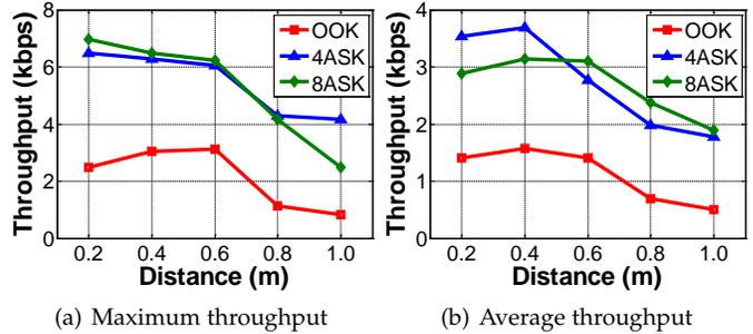
Fig. 15. Maximum and average throughput with a varying distance.
