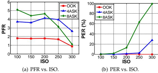
Fig. 8. PFR and PER with a varying ISO configuration.
