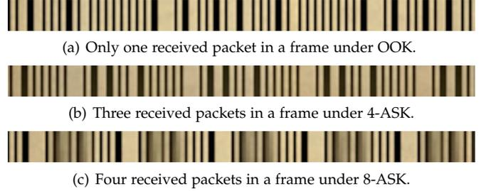
Fig. 7. Received packets in a frame under various CASK modulation.
