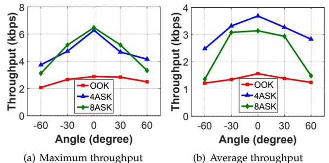
Fig. 16. Maximum and average throughput with a varying viewing angle.
