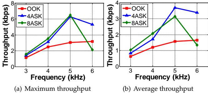
Fig. 14. Maximum and average throughput with a varying transmission frequency.
