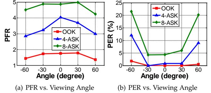
Fig. 12. PFR and PER under different viewing angle.
