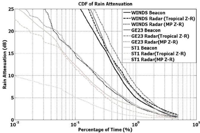
Fig. 5. Comparison of the CDFs of beacon measured attenuation and Radar calculated attenuation.
