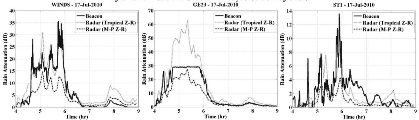
Fig. 3. Rain Attenuation during the Rain Event on 17 July 2010.
