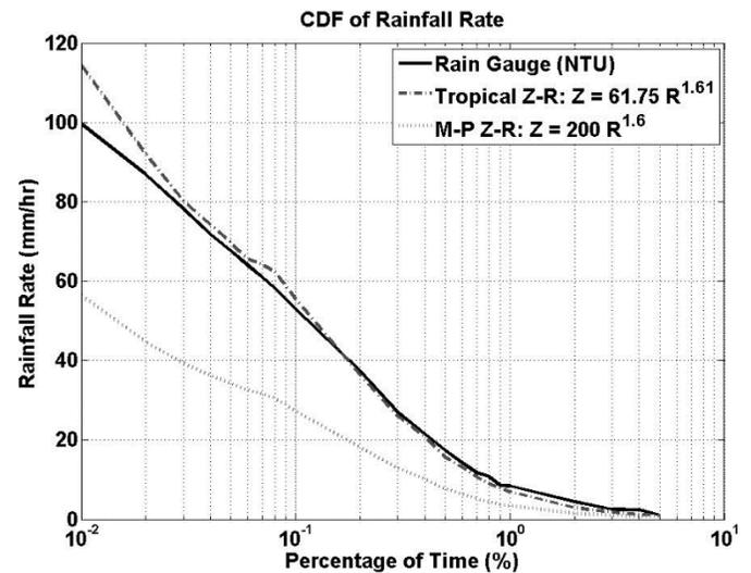
Fig. 1. Performance of tropical Z-R relationship on the Radar measured rainfall rate.
