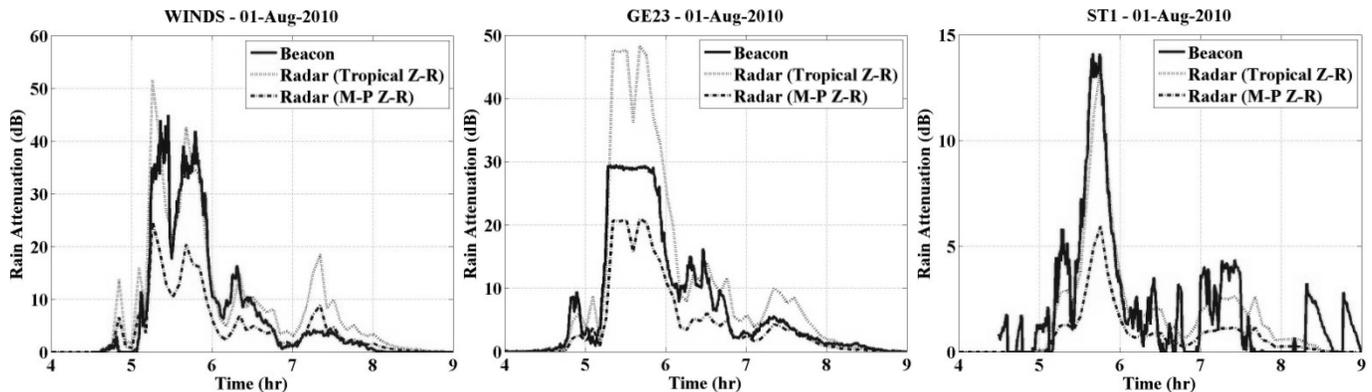
Fig. 4. Rain Attenuation during the Rain Event on 01 August 2010.
