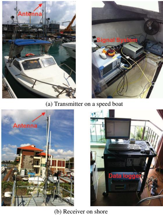
Fig. 1. Setup of transmission and data-logging systems for near sea-surface LoS measurements.
