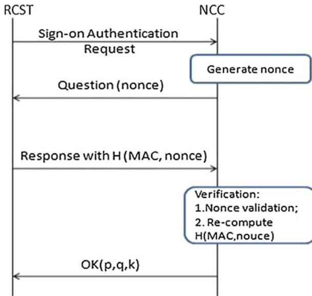
Fig. 4 ST sign-on authentication process with NCC
