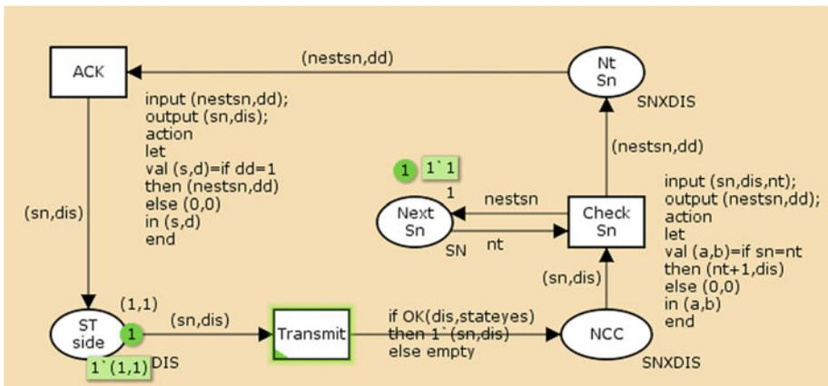
Fig. 6 CPN Model of normal transmission system
