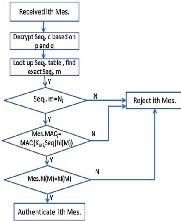
Fig. 5 Verification process of a received message
