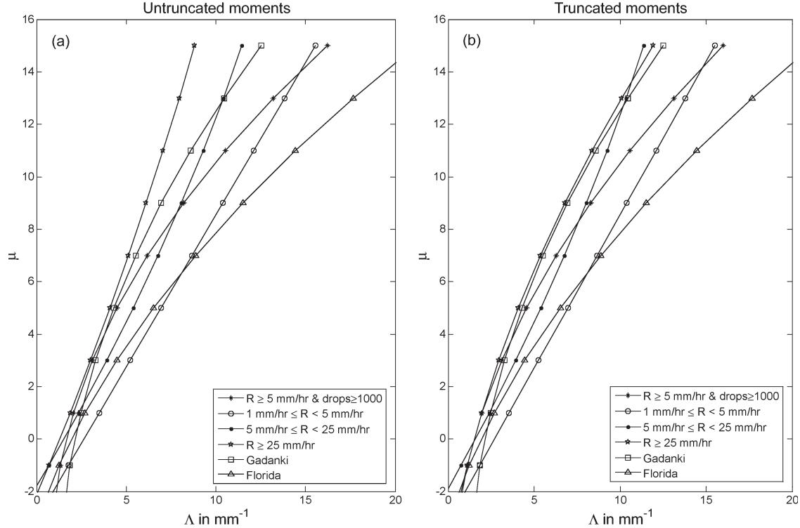
Fig. 6. Singapore's  $\mu$ - $\Lambda$  relationships for different rain categories, namely,  $R \geq 5 \text{ mm/hr}$  and *rain counts*  $> 1000$  drops,  $1 \text{ mm/hr} \leq R < 5 \text{ mm/hr}$ ,  $5 \text{ mm/hr} \leq R < 25 \text{ mm/hr}$ , and  $R \geq 25 \text{ mm hr}$ , along with Florida and Gadanki. (a) Untruncated moment method. (b) Truncated moment method.
