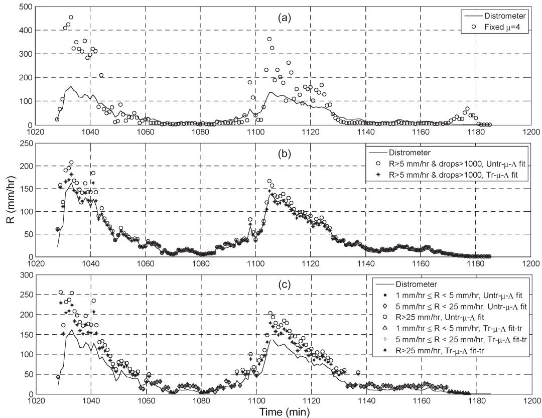
Fig. 7. Comparison of rain rates retrieved from polarimetric radar variables with measured rain rate for the rain event on February 26, 1995. (a) For  $\mu = 4$ . (b) Using the  $\mu$ - $\Lambda$  relation for the rain category  $R \geq 5 \text{ mm/hr}$  and *rain counts*  $\geq 1000$  drops. (c) Using the  $\mu$ - $\Lambda$  relations for the rain categories  $1 \text{ mm/hr} \leq R < 5 \text{ mm/hr}$ ,  $5 \text{ mm/hr} \leq R < 25 \text{ mm/hr}$ , and  $R \geq 25 \text{ mm hr}$ .
