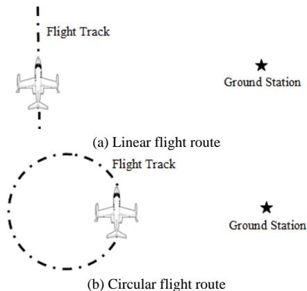
Fig.2. Two flight scenarios for the study of shadowing effect by maneuvering.
