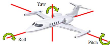
Fig. 1 Pitch, roll and yaw for an aircraft during maneuvering.
