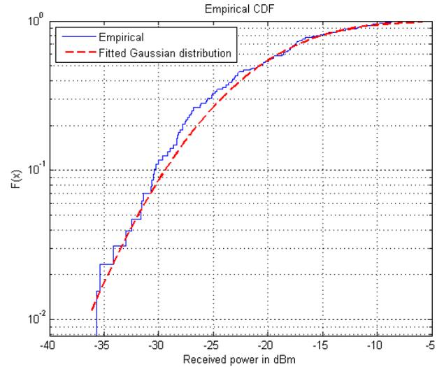
Fig. 6. CDF distribution of the received power for Channel 1 in the circular flight route
