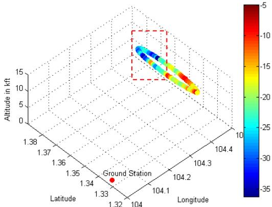
(a) Variation of the received power in 3-D geometry for Channel 1
