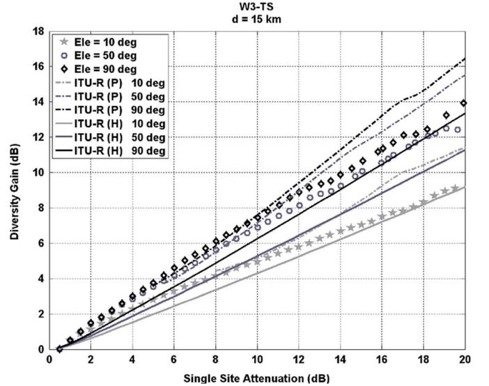
Fig. 5. Effect of Elevation Angle ( $F = 18.9$  GHz; Distance = 15 km; pol = V).
