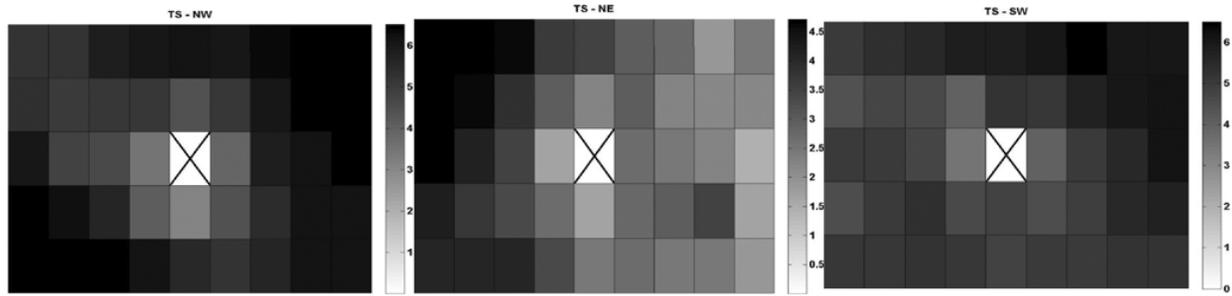
Fig. 11. Site Diversity gain of the rain events with different wind direction—Rain cell moves in the direction of the wind (Left: North-West; Middle: North-East; Right: South-West).
