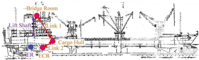
Fig. 1. Schematic drawing of antenna locations.
