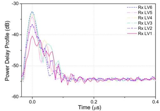
Fig. 2. Power delay profiles along the lift shaft at 2414 MHz.
