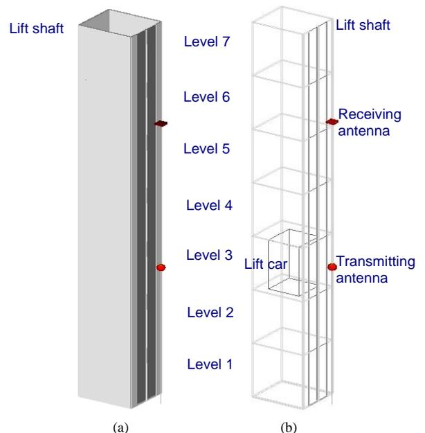
Fig. 7. Simulation scenario of the lift shaft in (a) solid view and (b) transparent view.
