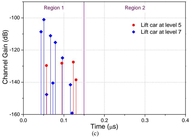
Fig. 11. Variation of lift car position. (a) Measured power delay profile. (b) Power delay profiles when lift car is at level 5 and at level 7. (c) Simulated ray tracing power delay profile.
