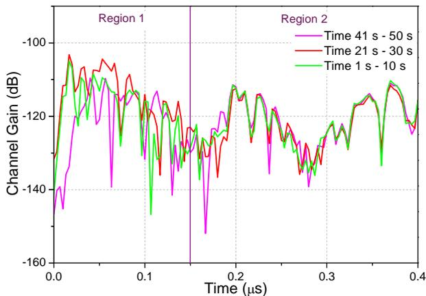
Fig. 10. Measured power delay profile when the lift car is moving.
