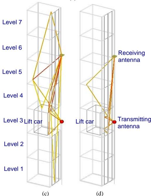
Fig. 8. Open-close lift door at transmitter level. (a) Measured power delay profile. (b) Simulated ray tracing power delay profiles. (c) 3D visualization from simulator for lift door open. (d) 3D visualization from simulator for lift door closed.
