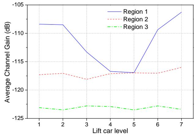
Fig. 13. Average channel gain for different lift car level.
