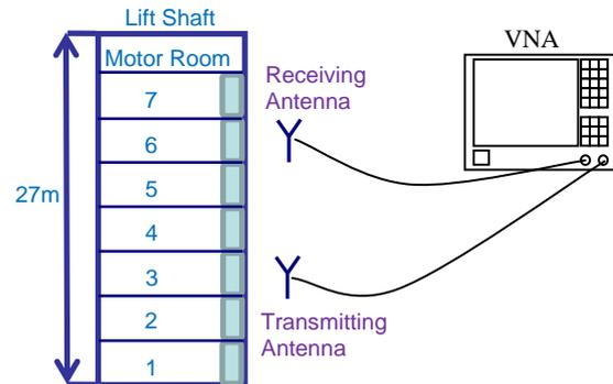
Fig. 2. Schematic diagram of the measurement setup.
