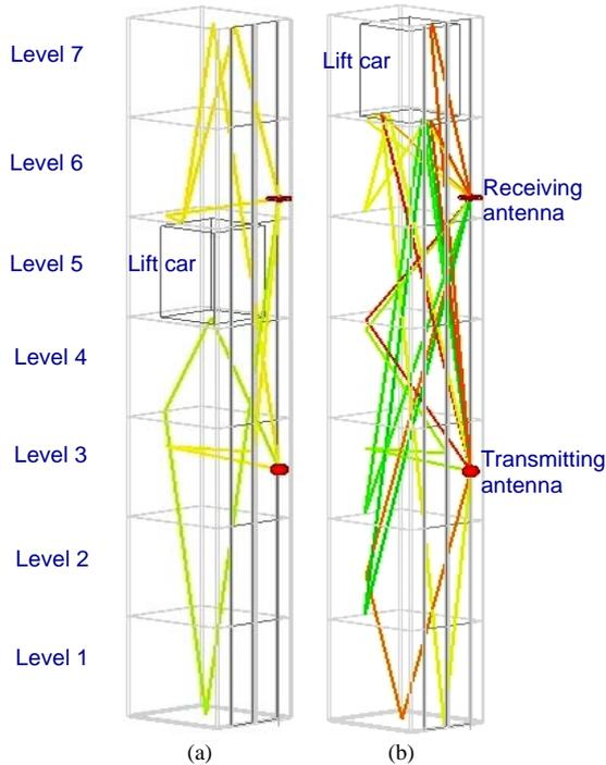
Fig. 12. Variation of lift car position. (a) 3D visualization from simulator for lift car at level 5. (b) 3D visualization from simulator for lift car at level 7.
