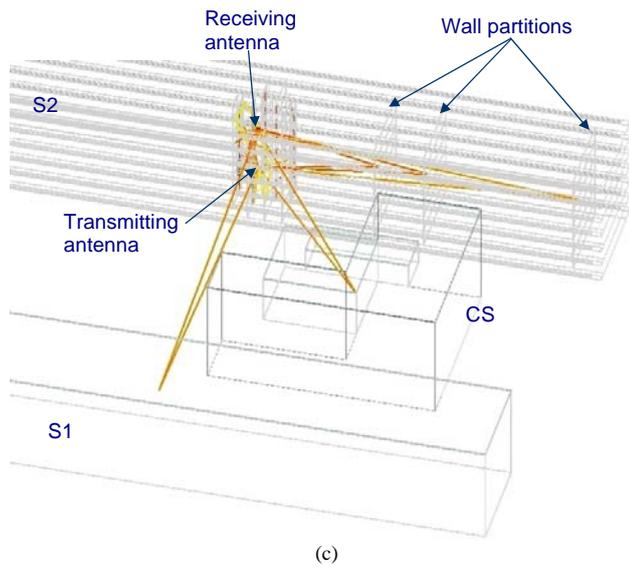
Fig. 4. (a) Measured power delay profile. (b) Simulated ray tracing power delay profile. (c) 3D visualization from simulator.
