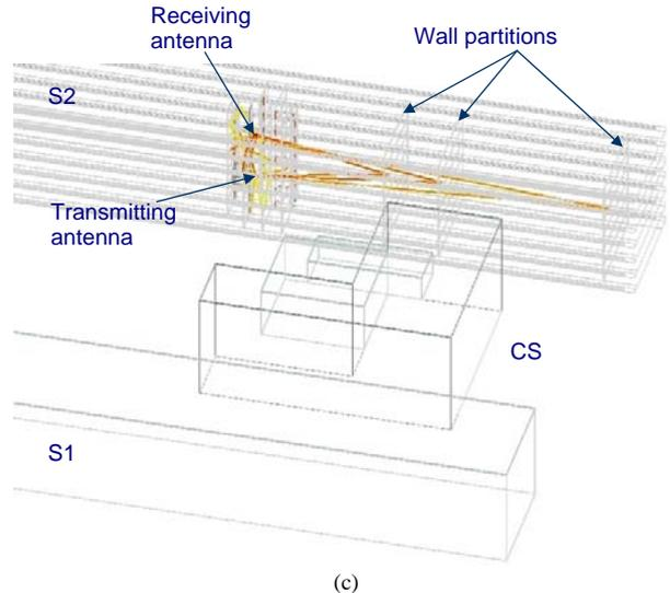
Fig. 5. Metallic plate at transmitter level. (a) Measured power delay profile. (b) Simulated ray tracing power delay profile. (c) 3D visualization from simulator.
