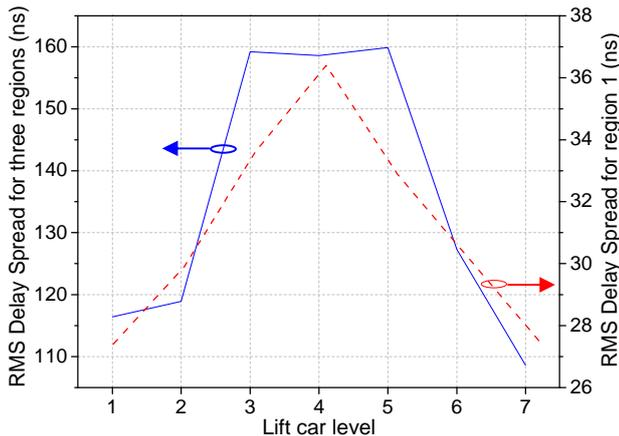
Fig. 14. RMS delay spread for different lift car level.
