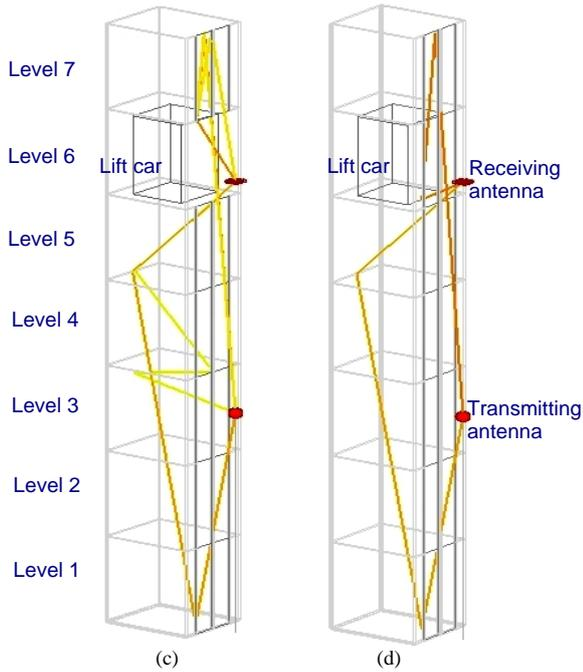
Fig. 9. Open-close lift door at receiver level. (a) Measured power delay profile. (b) Simulated ray tracing power delay profiles. (c) 3D visualization from simulator for lift door open. (d) 3D visualization from simulator for lift door closed.
