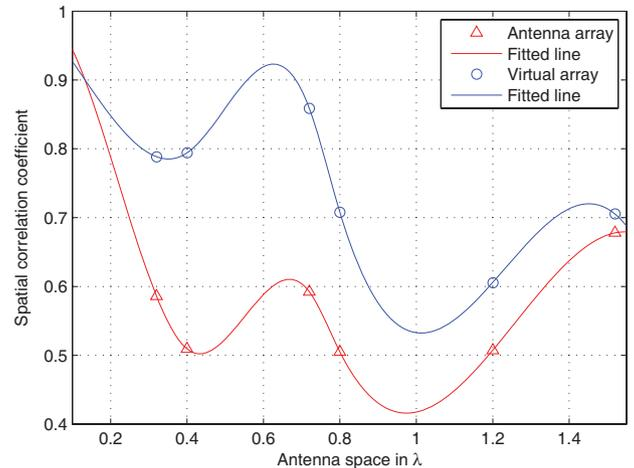
Fig. 1. Spatial correlation coefficients with different dual-receptor separation  $d$  at a forest depth of 710 m
