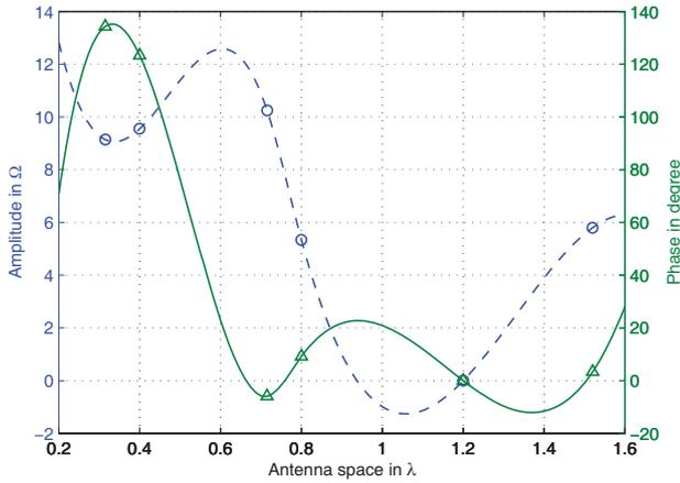
Fig. 2. The theoretical receiving mutual impedance with 50 Ω load; ---O--- Amplitude in Ω;—△—Phase in degree
