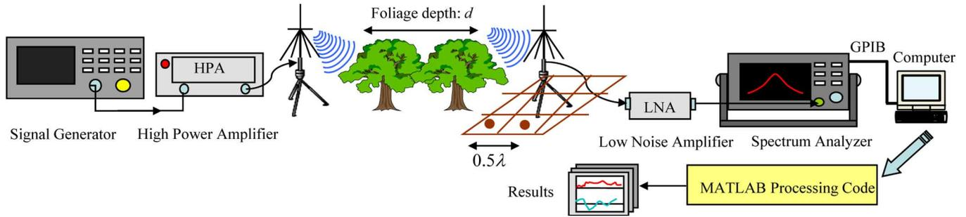
Fig. 3. The schematic diagram of measurement setup.
