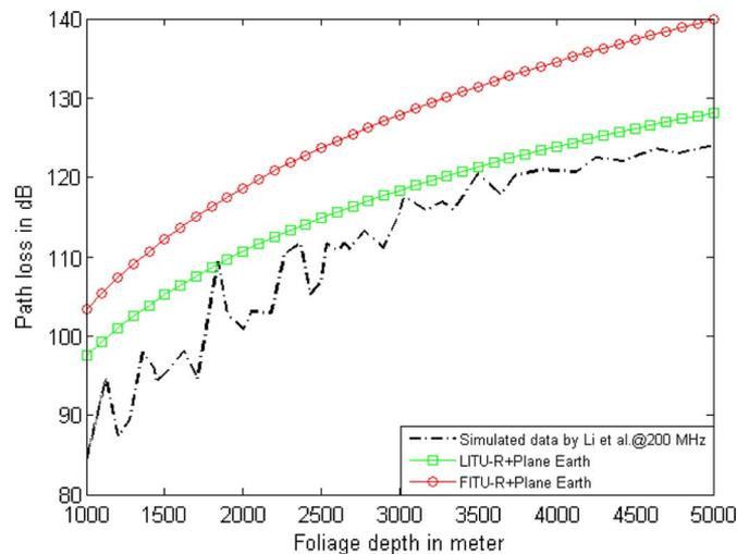
Fig. 7. Predicted path loss in forest at 200 MHz covering a long foliage depth of 1000–5000 m. Also shown are the simulated data by Li *et al.* [3].
