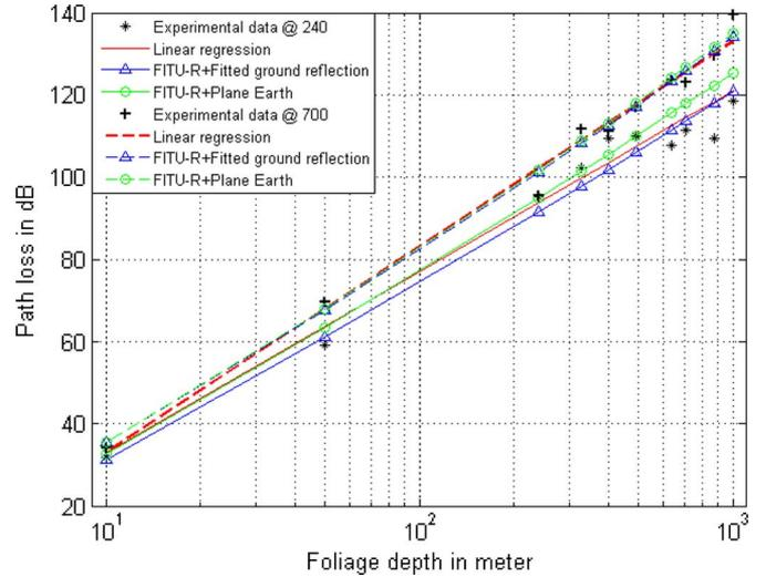
Fig. 5. Results with optimization of ground reflection.
