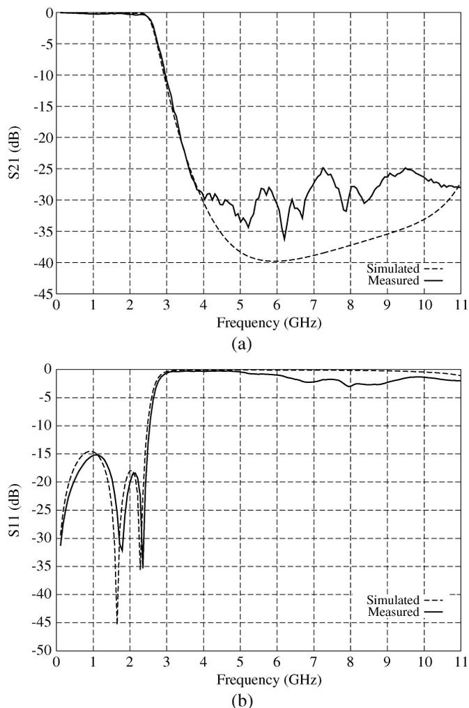
Fig. 8. Simulated and measured  $S$ -parameters of the proposed U-shaped DP-EBG microstrip low-pass filter structure. (a)  $S_{21}$ . (b)  $S_{11}$ .
