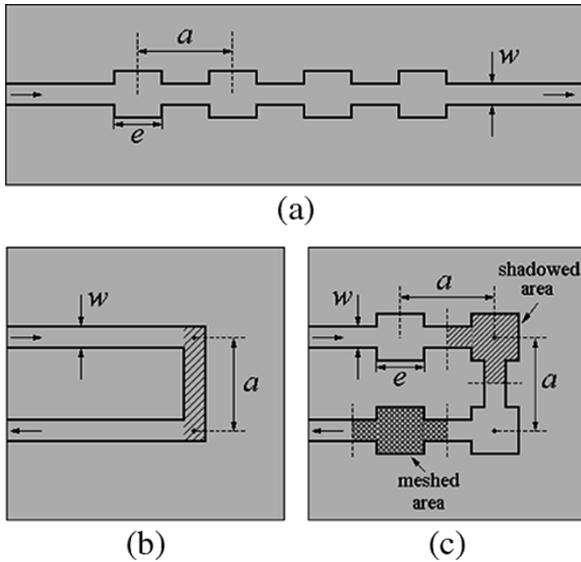
Fig. 1. Schematic of: (a) a straight EBG microstrip structure, (b) a U-shaped MLIN, and (c) a U-shaped EBG microstrip structure.
