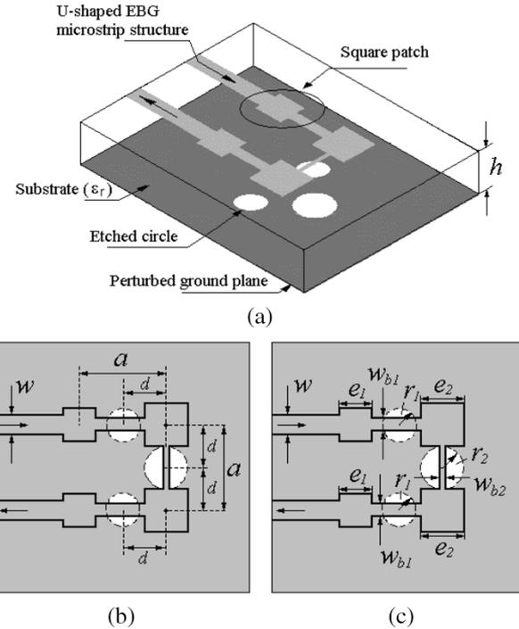
Fig. 5. Schematic of the proposed high-performance compact U-shaped DP-EBG microstrip low-pass filter structure. (a) 3-D view. (b) Top view 1. (c) Top view 2.
