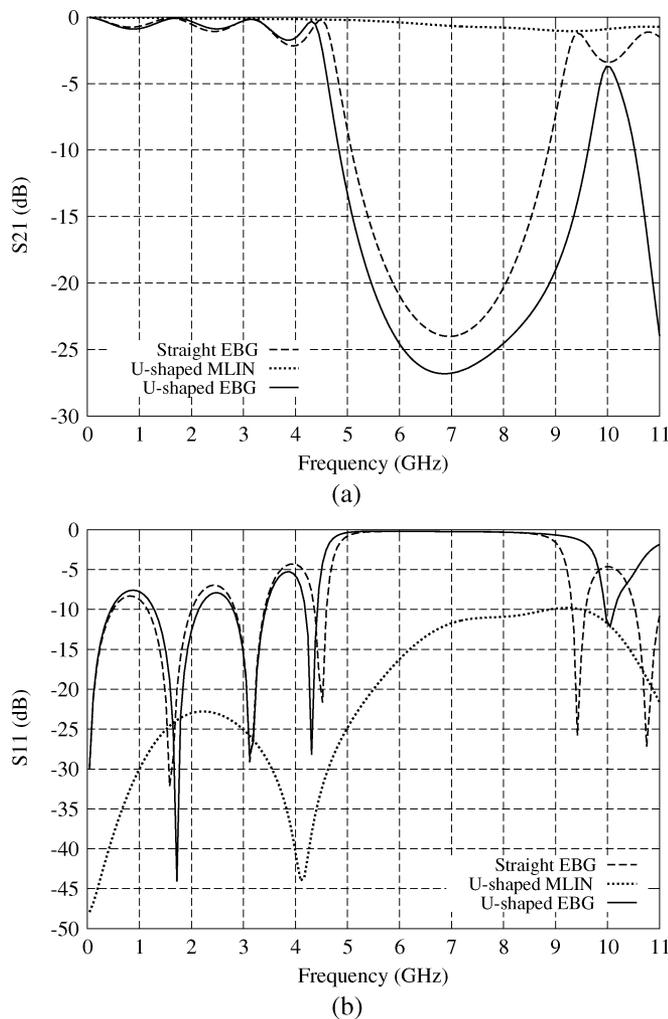
Fig. 2. Simulated  $S$ -parameters of structures in Fig. 1. (a)  $S_{21}$ . (b)  $S_{11}$ .
