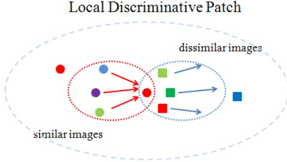
Fig. 2. The illustration of the Local Discriminative Patch for an image and its associated nearby similar and dissimilar images. Circular solid dots and square solid dots denote labeled similar and dissimilar images, respectively. For each given image, minimizing the objective function of the Local Discriminative Patch will pull the nearby similar images towards this image while pushing the nearby dissimilar images away from this image in the reduced subspace.
