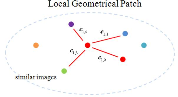
Fig. 3. The illustration of the Local Geometrical Patch for an image and its associated nearby similar images. Circular solid dots denote labeled similar images. For each given image, the Local Geometrical Patch aims to preserve the local geometry of labeled similar images before and after projection. Minimizing the objective function of the Local Geometrical Patch will reconstruct the given image from its associated nearby similar images with a minimal error in the reduced subspace.
