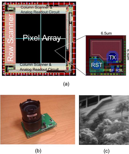
Fig. 7. (a) Layout of the proposed pixel architecture which has been embedded into a test chip. (b) Chip test platform which uses a FPGA system for chip controller and image readout. (c) Reproduced sample image
