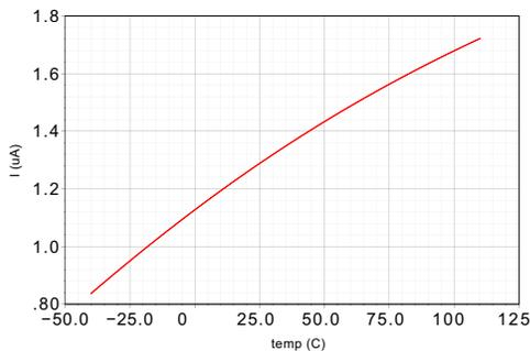
Fig. 4. Simulation result of the biasing current due to temperature change.
