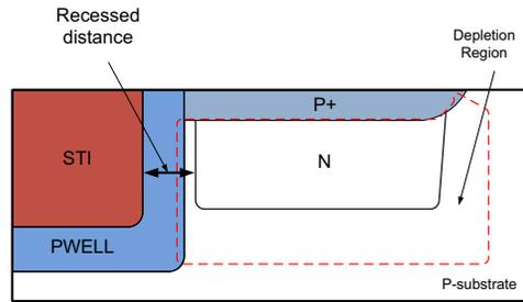
Fig. 3. Highlighted Cross-Sectional View of a Pinned Photodiode.
