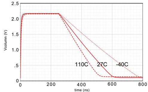
Fig. 5. Simulated waveform of the column bus showing the operation of charging and discharging under different temperature in a  $256 \times 256$  pixel array. The waveform denotes the worst-case readout scenario of two consecutive pixels with maximal voltage difference. The charging operation shows no significant difference. However, discharging through the biasing transistor is strongly affected under different temperature
