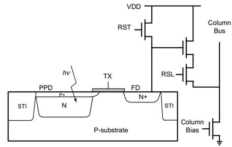
Fig. 1. Schematic and cross-sectional view of a typical 4T pixel architecture.
