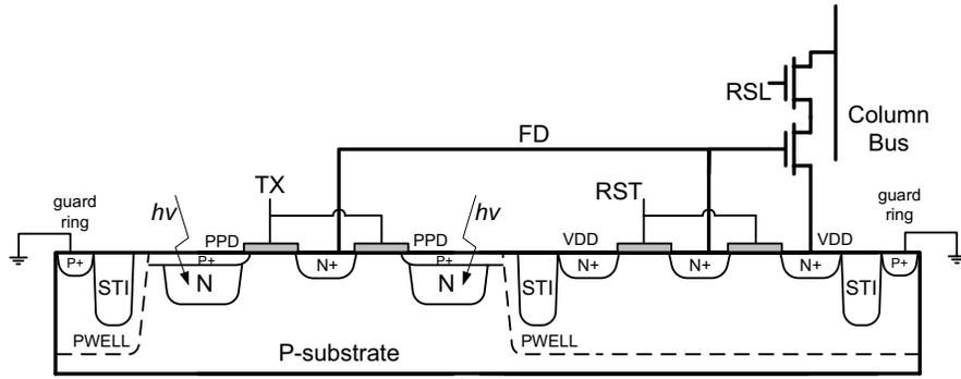
Fig. 2. Proposed radiation tolerant pixel architecture with its highlighted cross sectional view of the pinned photodiode and floating diffusion node.
