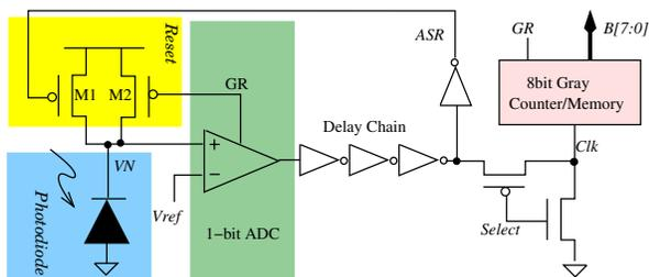
**Fig.1** – In-pixel building blocks
