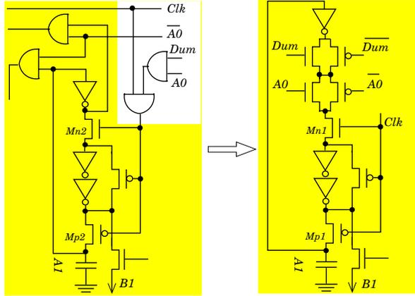
**Fig.5** – Improved implementation using transmission gates for B1.
