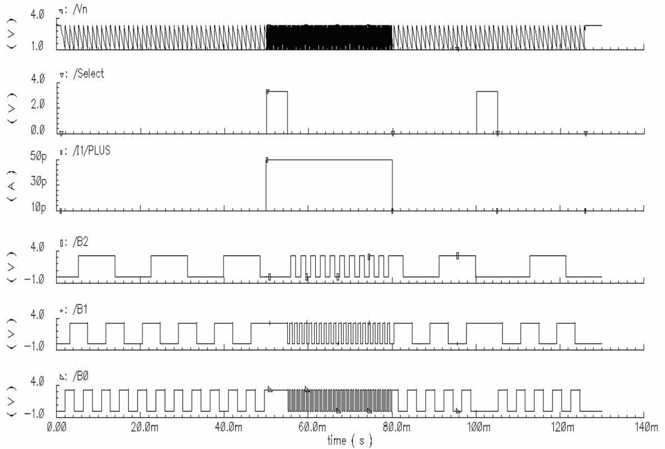
**Fig.4** – Gray code counter memory: simulation results
