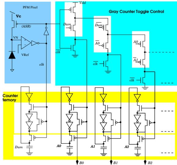
**Fig.6** – Counter memory structure implemented using domino
