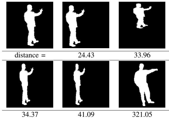
Fig. 5. Simulation results of size and position invariance recognition. The top left image is an original reference, the rest ones except the last figure are obtained by either position shifted, vertically or horizontally scaled. The line segment Hausdorff distance between the first image and reset ones were calculated and shown under each image.
