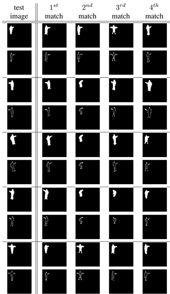
Fig. 6. Simulation results of human posture recognition. The first column is the test image while the right four columns are library images ranked by similarity. For every two rows, the first row shows the raw image acquired by the Octopus imager plus IFAT processor, while the second shows the corresponding S1 layer image.
