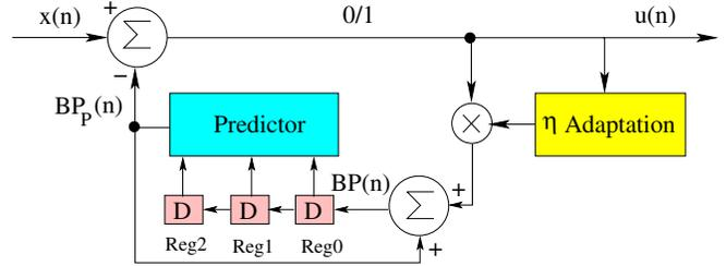
Fig. 2. 1-bit Adaptive Q combined with DPCM.
