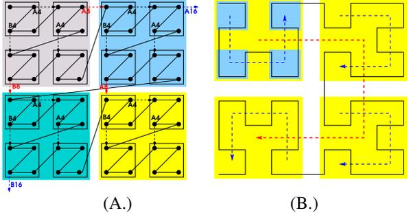
Fig. 3. (A.)Smooth boundary point propagation scheme using Morton (Z) scan. (B.)Hilbert scan patterns at each hierarchy for an  $8 \times 8$  array.
