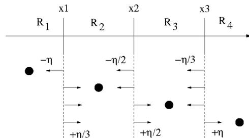
Fig. 1. Example of the backward adaptation  $FBAR_0$  for a 2-bit quantizer.
