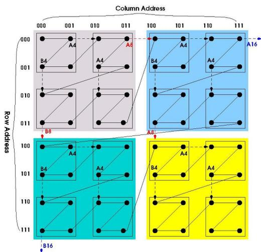
Fig. 2. Smooth boundary point propagation scheme for  $4 \times 4$  and  $8 \times 8$  pixel quadrants. Two registers ( $A4$ ,  $B4$ ) are needed to store the boundary point for the  $4 \times 4$  quadrant level and two other registers ( $A8$ ,  $B8$ ) are needed to store those related to the  $8 \times 8$  quadrant level.
