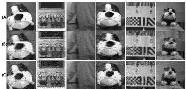
Fig. 7. Captured images under different processing modes. Row (A.) shows the 8-bit captured images without compression, (B.) and (C.) represent the reconstructed compressed images using 1-bit adaptive quantizer with fixed  $\eta$  raster scan, 1-bit adaptive quantizer using adaptive  $\eta$  smooth boundary Morton(Z) scan, respectively.
