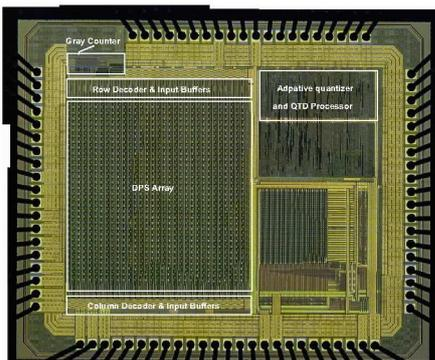
Fig. 6. Microphotograph of the prototype Chip.
