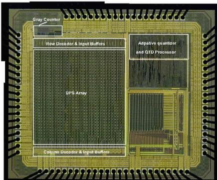
Fig. 6. Microphotograph of the prototype Chip.
