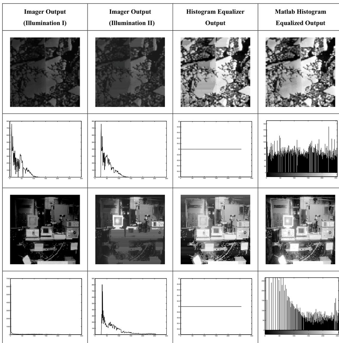
Fig. 5. Output of the AER imager. Column 1 and column 2 are images acquired at two different illuminations. Column 3 and 4 are the histogram equalization outputs from the imager and Matlab simulation, respectively.
