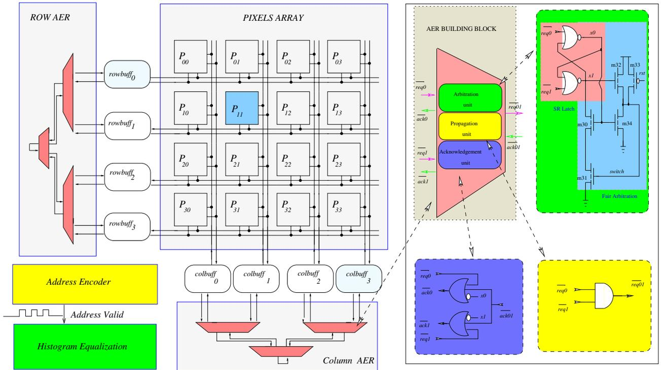
Fig. 2. Vision Sensor Architecture
