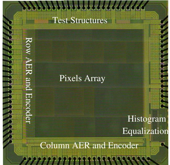
Fig. 4. Microphotograph of the chip.
