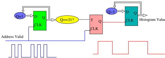
Fig. 3. Histogram equalization circuitry
