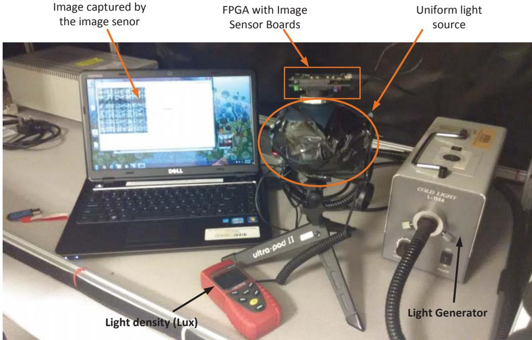
Figure 4.23: Setup of image performance testing.
