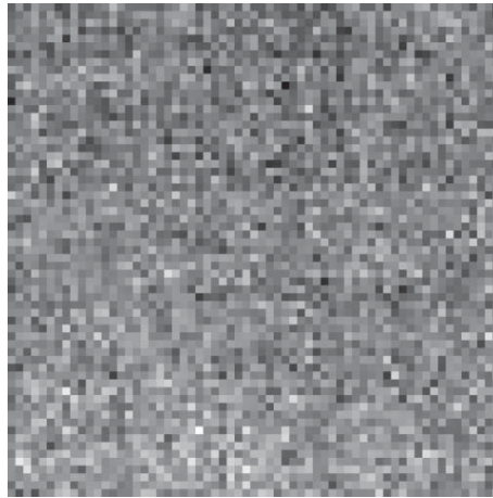
Figure 5.1: A typical FPN image of a CMOS image sensor [14].
