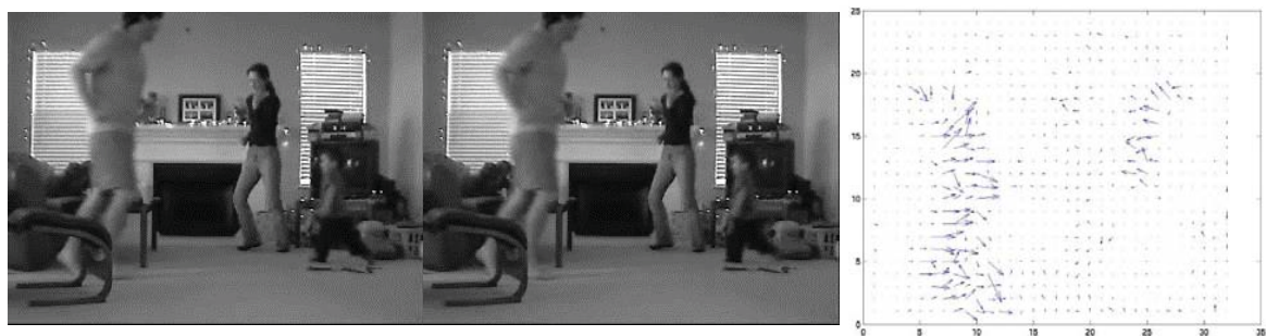
Figure 2.8: Optical flow descriptors using Horn and Schunck method [78]. Given image sequence from the first to the second, optical flow is then calculated showing in the third image
