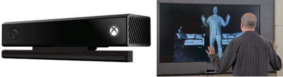
Figure 2.2: Depth sensor using in Microsoft XBOX Kinect (left) and its captured images (right) [29]
