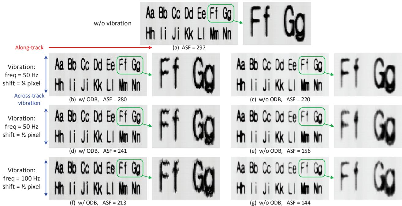
Fig. 17. Sample TDI images without vibration and with vibration (including variable levels and frequencies).
