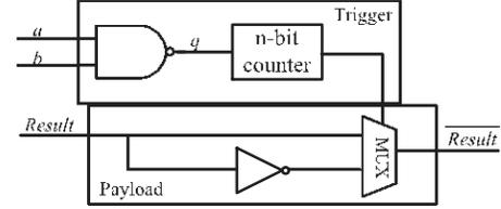
Fig. 12. Counter-based Trojan circuit architecture [35].
