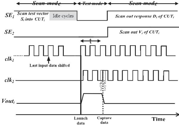
Fig. 11. Timing diagram of the sampling of transition delay.
