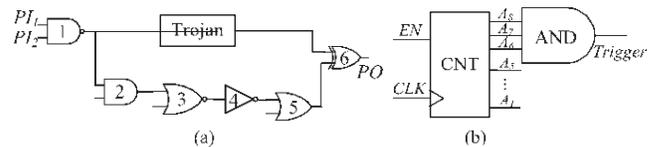
Fig. 1. Example of a HT (a) with no delay impact, (b) with no switching power impact.
