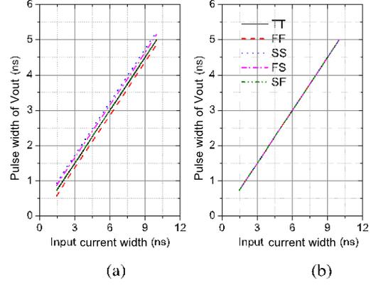
Fig. 8. Corner simulation of comparator output pulse width: (a) without calibration, (b) with calibration. The process corner is represented by a two-letter designator, where the first and second letters refer to the NMOS and PMOS corners, respectively. The letters T, F and S denote typical, fast and slow corners, respectively.
