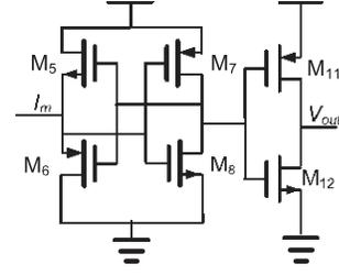
Fig. 7. Schematic of Traff's current comparator [31].
