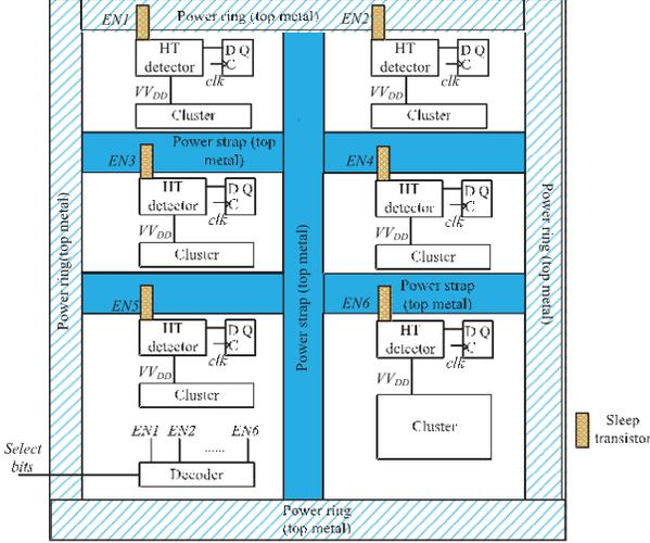
Fig. 4. Example of the deployment of the proposed HT detector with six virtual-power clusters.
