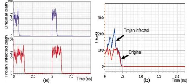
Fig. 3. Supply current waveforms for the sensitized path of Trojan-free and Trojan-infected circuits: (a) the Trojan is inserted in series, (b) the Trojan is inserted in parallel.
