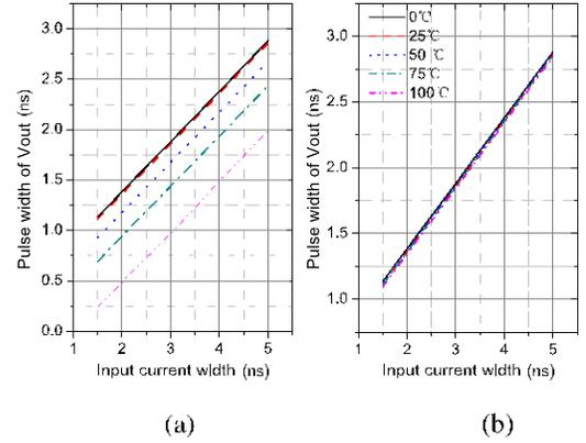
Fig. 9. Simulation of comparator output pulse width under temperature variations: (a) without calibration, (b) with calibration.
