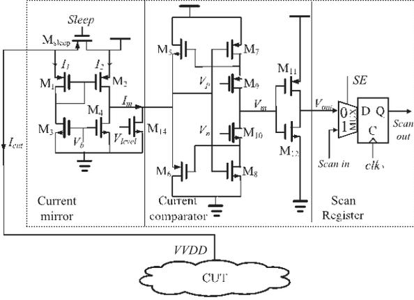
Fig. 6. Schematic of the proposed current sensing to path delay monitoring circuit.
