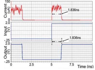
Fig. 2.  $I_{DDT}$ , input and output waveforms due to a sensitized path in C432.
