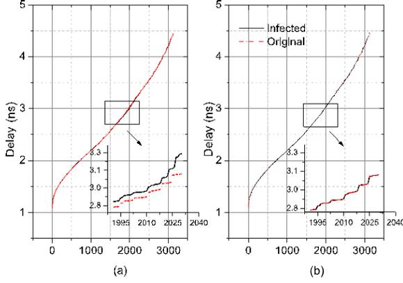
Fig. 14. The delay impacts with different placements of Trojan: (a) Trojan embedded in serial, (b) Trojan embedded in parallel.
