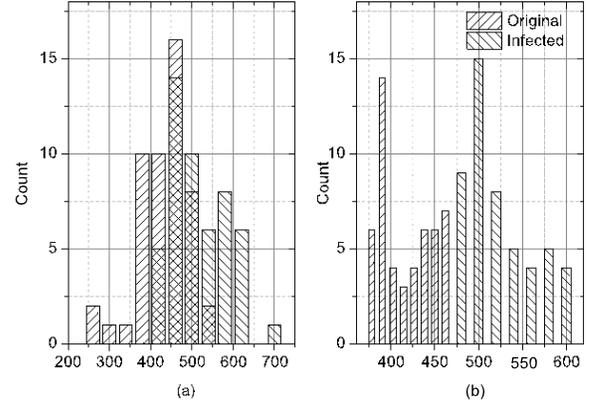
Fig. 13. Monte Carlo simulation results for the active current duration distributions: (a) before calibration, (b) after calibration.
