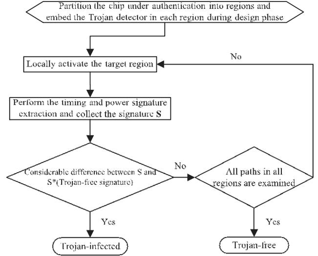
Fig. 5. The HT detection flow using the proposed HT-detector.
