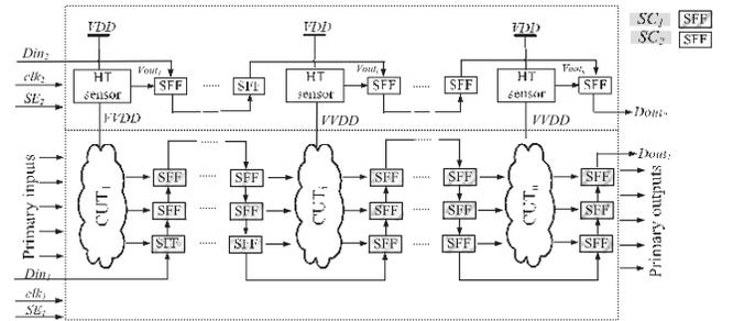
Fig. 10. Primary and secondary scan chains for the detection of current comparator output pulse width.
