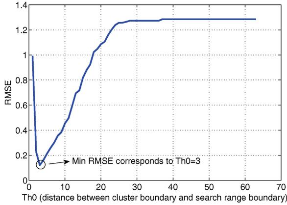
Fig. 6. RMSE versus  $Th0$  for a test image sequence (given three clusters). The optimal  $Th0$  is 3.
