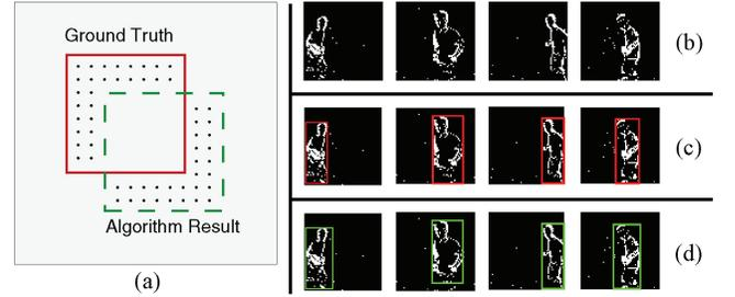
Fig. 5. (a) Figure that is used to illustrate the definition of localization error. Dotted regions represent the nonoverlapping area. (b) Lists some sample test images. (c) and (d) present corresponding ground truth and simulation results (at certain  $Th_0$  and number of clusters), respectively.
