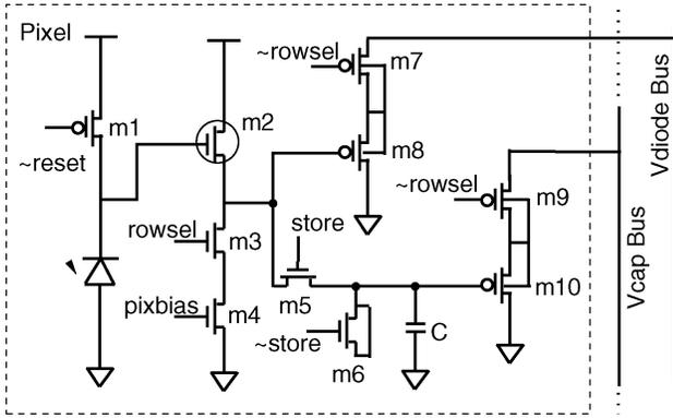
Fig. 11. Schematic of the pixel. Low threshold NMOS follower m2 is highlighted with a circle. Capacitor C is the memory device that stores the previous-frame pixel value.
