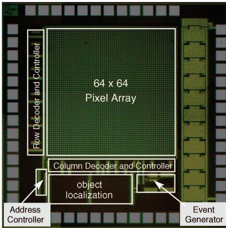
Fig. 16. Chip microphotograph with main building blocks highlighted.
