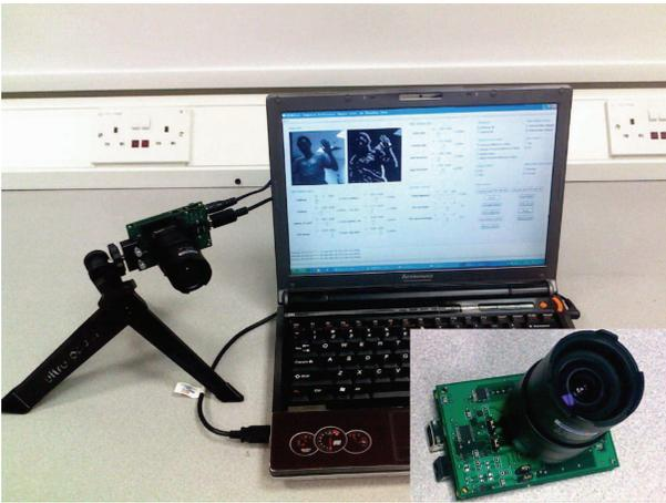
Fig. 17. FPGA based testing platform. The vision sensor is interfaced with an Opal-Kelly XEM 3005 FPGA board.
