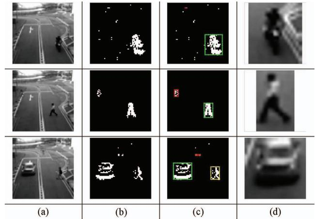
Fig. 18. Sample images of the prototype image sensor. (a) Gray level images captured in normal intensity mode. (b) Corresponding images captured in temporal difference mode. (c) Localization results on top of the temporal difference images. (d) Snapshot of the ROI (images are resized in software for better visualization).
