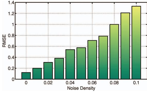
Fig. 9. RMSE versus noise density. (Algorithm parameters: three clusters, search range threshold  $Th_0$  equals 3.)
