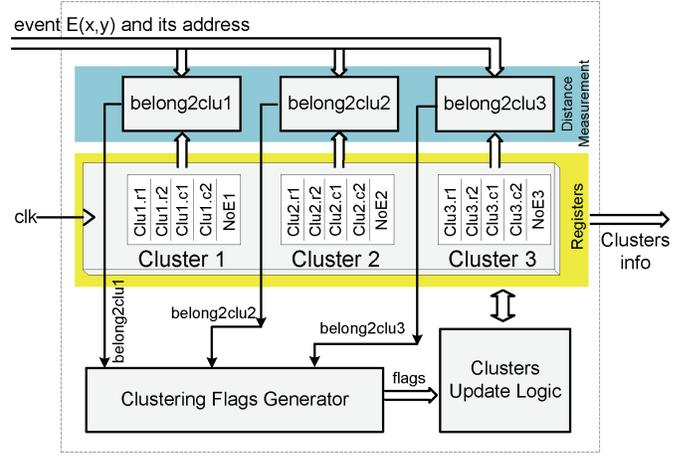
Fig. 12. Block diagram of the object localization unit.
