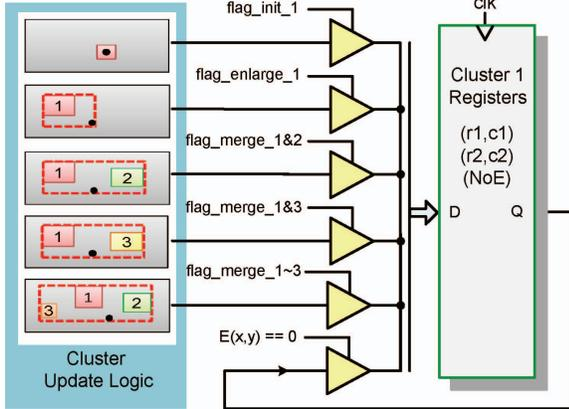
Fig. 15. Update of cluster-1 registers. Clustering flags control a series of tri-state buffers to choose the right boundary update results.
