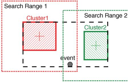
Fig. 3. Illustration of instant merging. If the incoming event belongs to more than one cluster at the same time, then all corresponding clusters and current event will be merged together.
