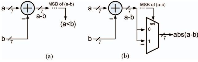
Fig. 13. Arithmetic operations for  $(a < b)$  and  $abs(a - b)$ . (a)  $(a < b)$ . (b)  $abs(a - b)$ .
