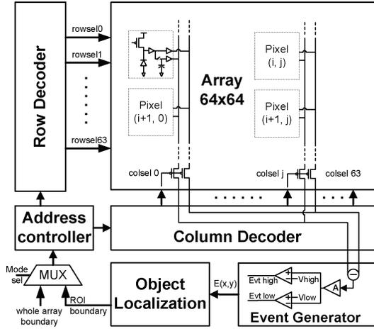
Fig. 1. Block diagram of the single-chip image sensor with moving objects detection and localization functionality. The event generator digitalizes temporal differences into sequential motion events, which are processed by the moving object localization unit on the fly to find the boundary addresses of the moving object region. With these addresses, the address controller enables the image sensor to extract the image in the ROI.
