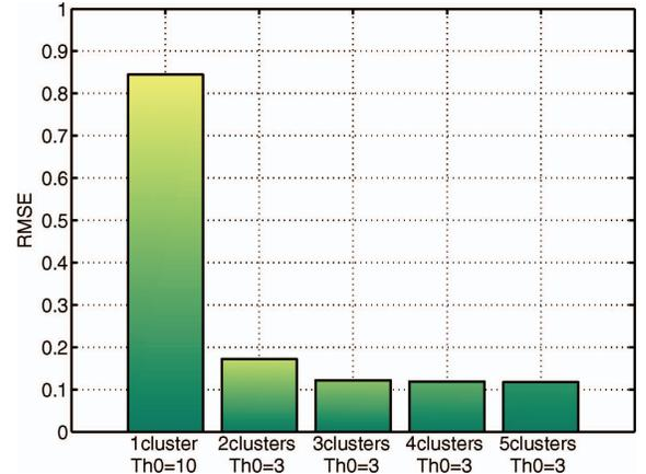
Fig. 7. RMSE versus number of clusters (at corresponding best threshold  $Th0$ ). Three clusters are enough for the given test image library.
