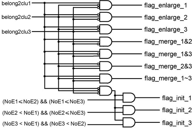
Fig. 14. Generation of the clustering flags. The 3 bits of comparison results (“belong2clu1,” “belong2clu2,” and “belong2clu3”), together with the information of NoE in each cluster, generate ten clustering flags.
