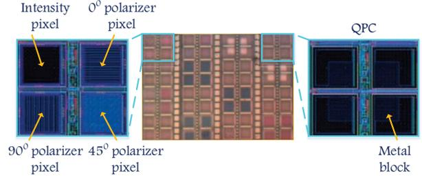
Fig. 5. Microphotograph of the pixel array along with the layout of polarization and QPC pixels.
