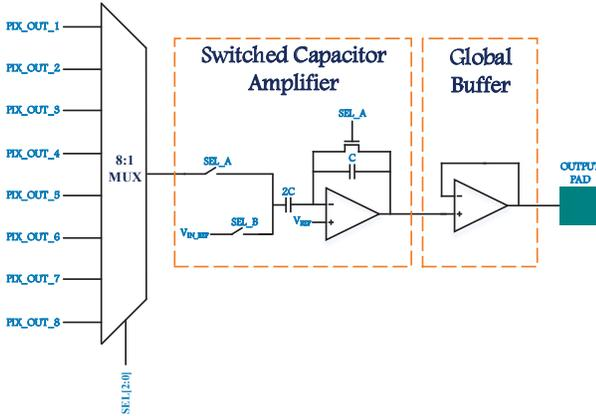
Fig. 4. Figure illustrating signal data path to the output pad.
