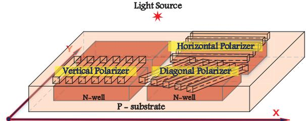
Fig. 2. Physical structure of a group of polarization pixels with different polarizer orientations.
