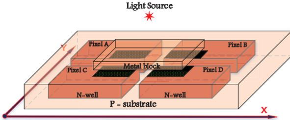
Fig. 1. Physical structure of a quadrature pixel cluster.
