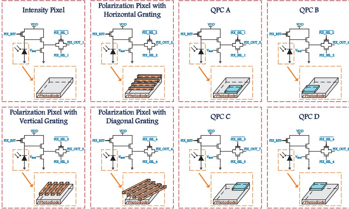
Fig. 3. Pixel-unit-cell comprising of an intensity pixel, three polarization pixels and a quadrature pixel cluster.
