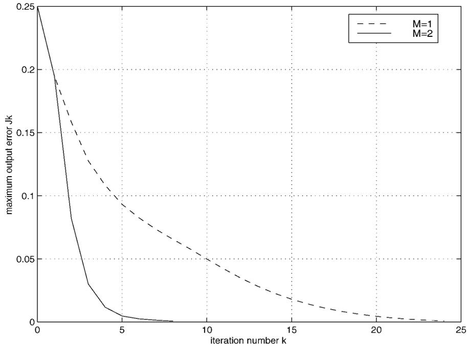
Figure 1. Convergence rate comparison for  $M = 1, 2$  in the absence of resetting errors.
