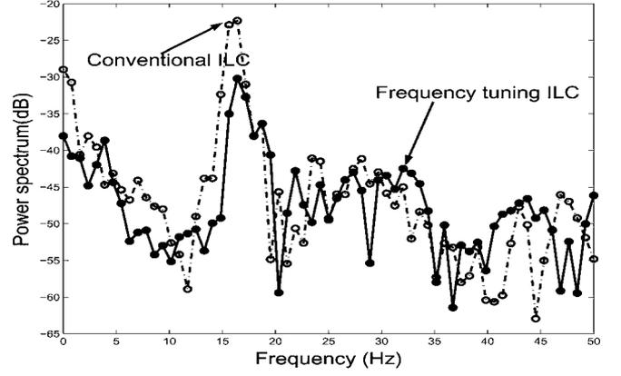
Fig. 13. Power spectrum comparison.
