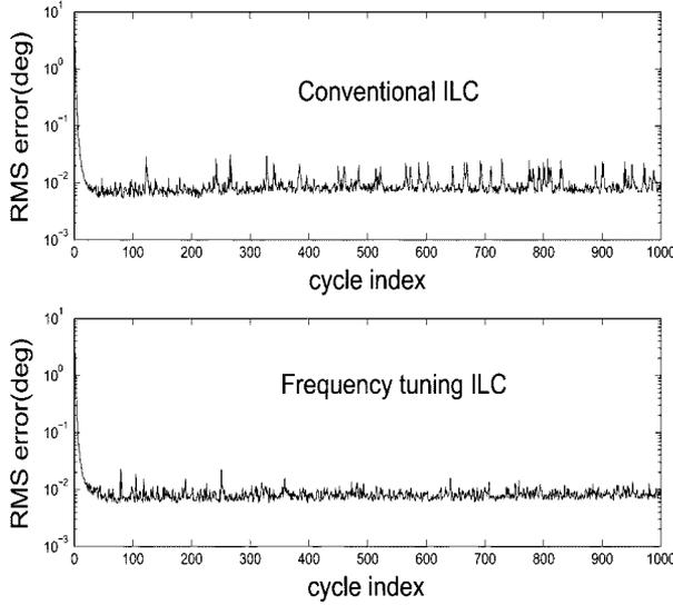
Fig. 9. RMS error of lead-step 5 and cutoff 15 Hz.
