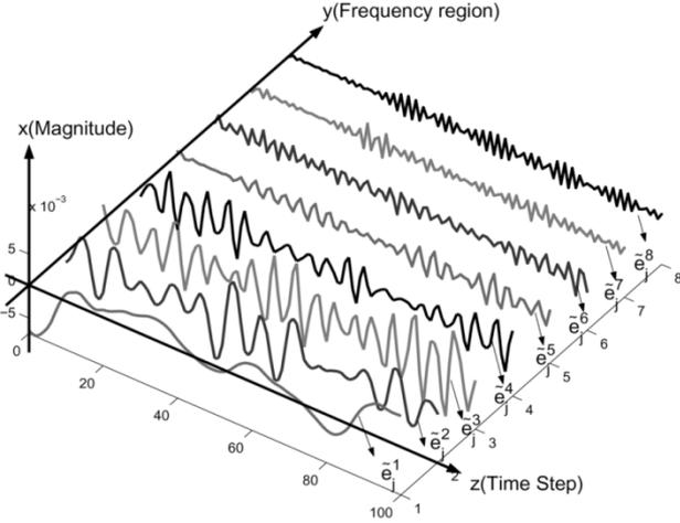
Fig. 2. Wavelet decomposition of error signal.
