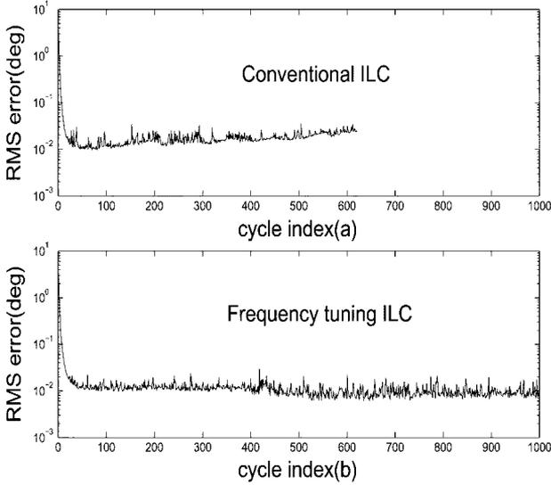
Fig. 12. RMS error of lead-step 5 and cutoff 17 Hz.
