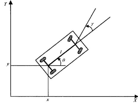
Figure 2: Pictorial of a car-like robot
