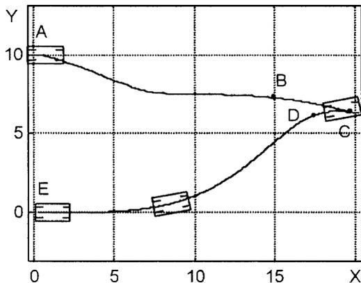
**Figure 3:** Parallel parking control of a car-like robot: Cartesian motion
