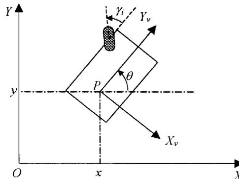
Figure 1: A mobile robot with steerable wheels
