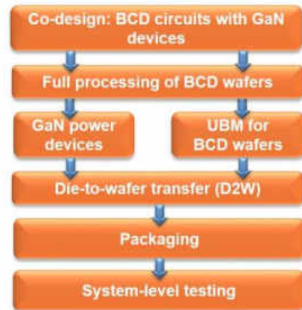
Fig. 2 Design flow of the GaN2BCD™ technology.
