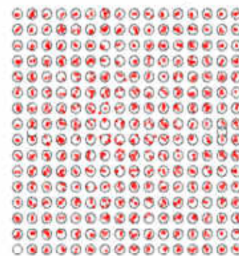
Constellation of 256-QAM with EVM of -32.5dB at 5.53 GHz
