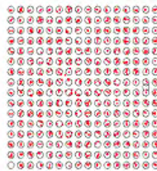
Constellation of 256-QAM with EVM of -32.5dB at 5.53 GHz
