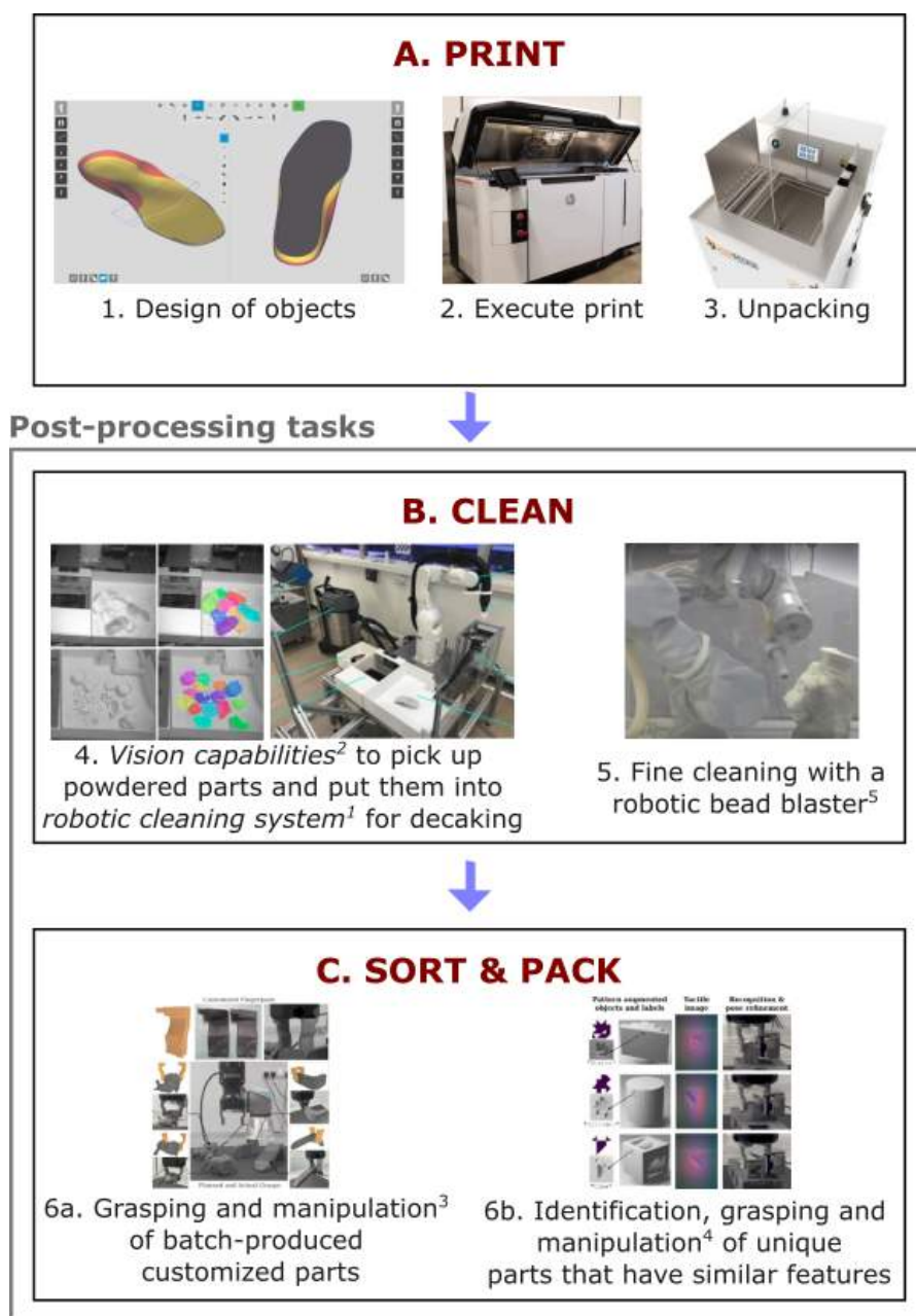
FIGURE 7.1: Illustration of possible integration of different contributions in three stages of 3DP: (A) Print; (B) Clean; and (C) Sort and Pack. Post-processing tasks would begin after printing.
