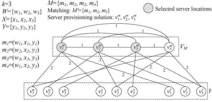
Fig. 2. Example instances of the 3DM problem and the DIA server provisioning problem
