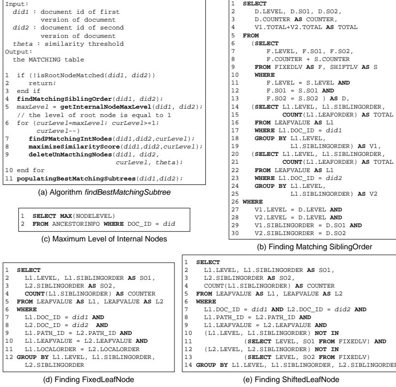
Fig. 7. Bottom Up Approach: Algorithm BU-findBestMatchingSubtree and SQL Queries.
